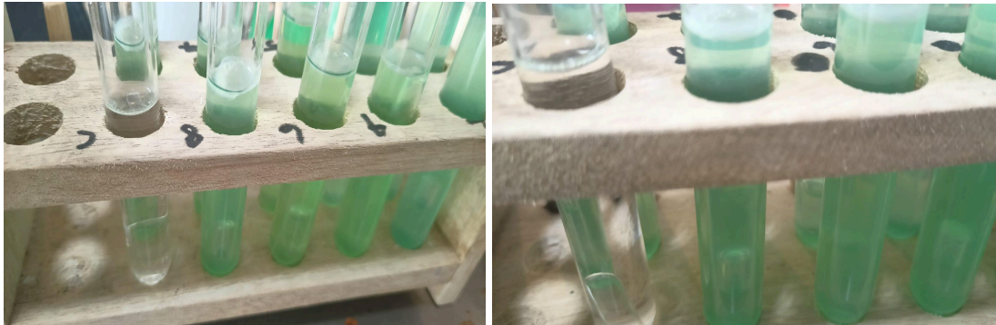
Figure 7. Laboratory Analysis Results Showing Bubbles in Durham Tubes Indicating Coliform and Fecal Coli Bacteria
