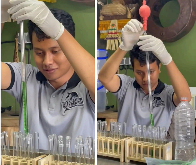
Figure 5. Preparation of LB and BGLB Solutions with Distilled Water and Seawater
